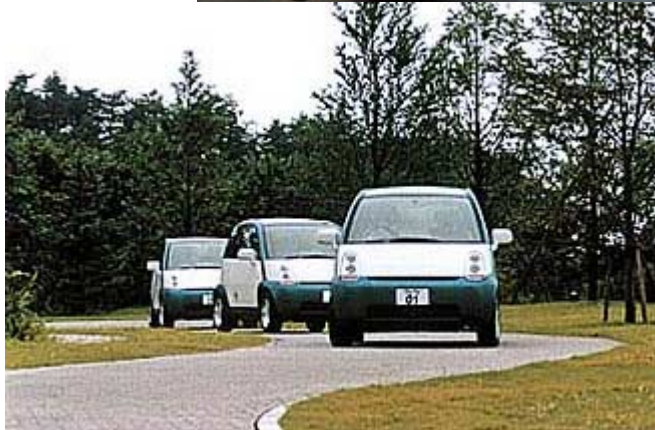
ICVS-City Pal, Platoon Drive (unmanned driving) from a station to another station
